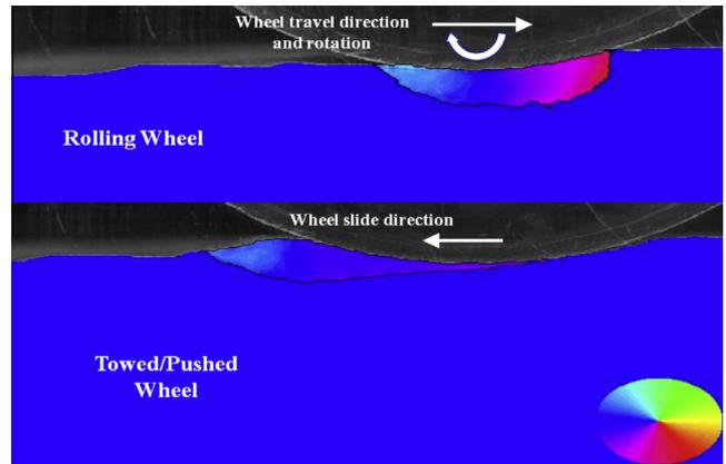
Fig. 4. Soil directional response to rolling wheel vs. pushed wheel; color indicates direction of soil particle velocity (Moreland et al., 2011). (For interpretation of the references to color in this figure legend, the reader is referred to the web version of this article.)
