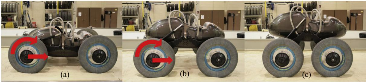
Fig. 1. Scarab going through inching procedure: (a) at its greatest wheel base, (b) mid position, and (c) smallest wheel base.
