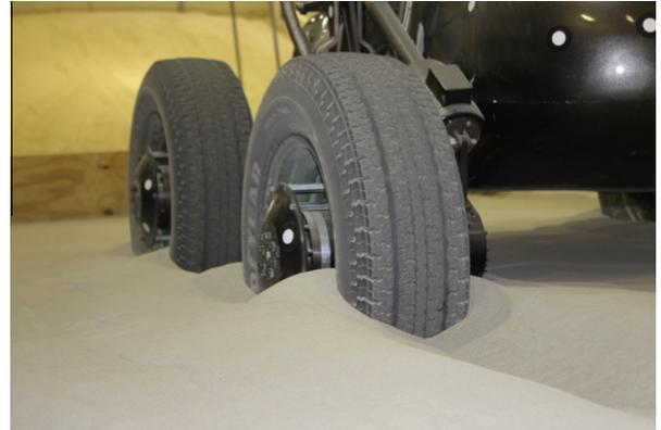
Fig. 6. Pneumatic rubber tires buried in Fillite.
