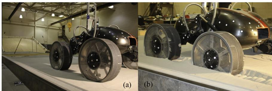
Fig. 7. The Scarab rover with rigid tires (a) before beginning driving and (b) while driving in the Fillite.
