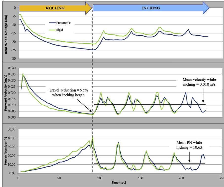
Fig. 13. Results of the Scarab rover driving using conventional rolling for 90 s, then inch-worming.
